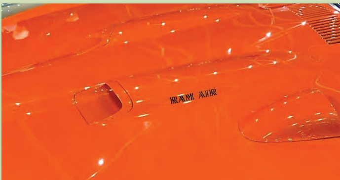
Figure 1. The Ram Air decals on this 1969 Judge are too close to the driver and not in the position the factory intended.
