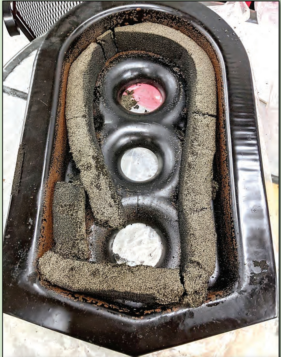
Figure 1. A photo of an NOS 1965 Ram Air pan and gasket. Since both came in the same box it was purchased over the counter as an accessory package (part number 984716 called an “air inlet package”). The pan and the foam could be purchased under their respective part numbers at the parts counter as well. Note that the deteriorating foam is not glued to the pan and there is no evidence that it ever was. The purchaser had to do that.
